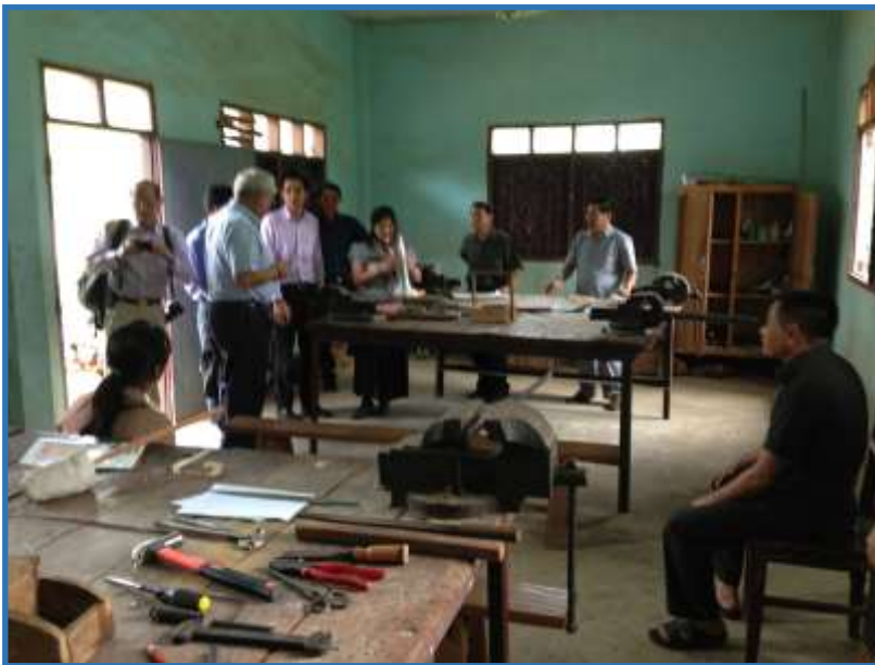
The 686 team and workshops were equipped to deal with conventional metal prostheses and orthoses, thermoplastics (polypropylene) and laminations, but needed Local Exhaust Ventilation for resin fumes.
